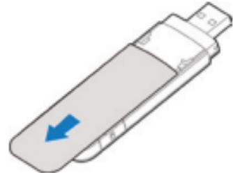
2. Insert the SIM card into the SIM card slot.
