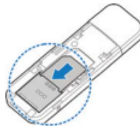
3. Insert the microSD card into the microSD card slot.
